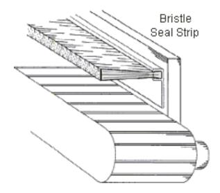
In one application, empty boxes tended to tumble down an incline; side brushes controlled motion and position with slight pressure on the boxes' sides as they moved down the conveyor.
