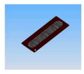
Ribbon is placed onto a thin, premade, diecut or molded plastic part and sonic welded in place.
