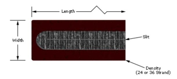
MultiFlex<sup>TM</sup> is generally used as a flexible sight seal or splashguard where the mounting surface is irregular such as being curved or wavy. MultiFlex<sup>TM</sup> begins with a ribbon of fill material that can be attached in several ways to various materials to form the final brush.
